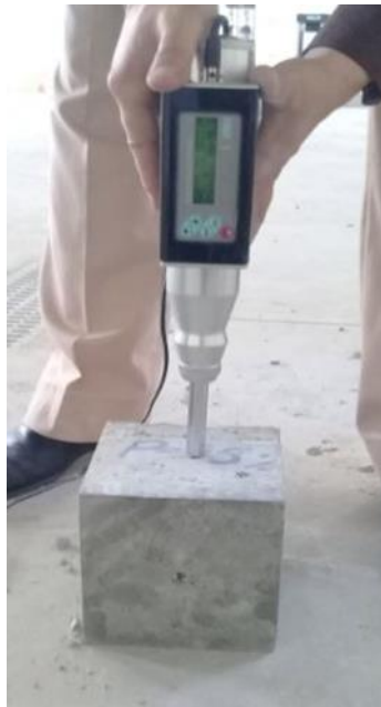
Figure 2.9 Rebound hammer test
